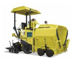
The machine has three axles: front, two axles for steering and rear, axle for traction. The rear axle is fitted with large pneumatic tyres so that the machine can be driven also on soft grounds. The actual version is equipped with four wheel drive traction as a standard. The steering system with a hydraulic pump gives a smooth control when turning. The hoppers are independently controlled by an electric-hydraulic system. The front pushing
