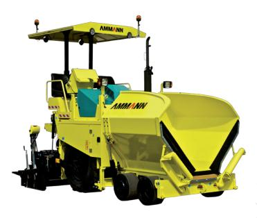
The machine has three axles: front, two axles for steering and rear, axle for traction. The rear axle is fitted with large pneumatic tyres so that the machine can be driven also on soft grounds. On the front oscillating axles are fitted large full rubber tyres. The steering system with a hydraulic pump gives a smooth control when turning. The hoppers are independently controlled by an electric-hydraulic system. The front pushing rollers move in
